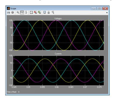
In "Build a Simple Three-Phase Model" on page 3-2, the electrical characteristics of three-phase load are purely resistive. In this model, the **Component structure** parameter of the RLC block is set to Series RL,
